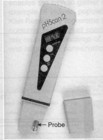
pH meter: Measures the acidity of water or soil, if it is first dissolved in pure water (pH scale 0 to 14).
