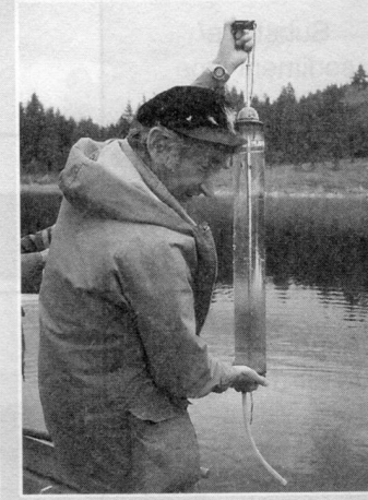
Collecting a water sample: A Nansen bottle is used to collect water samples from a lake for lab analysis, testing for nutrients, oxygen and pH.
